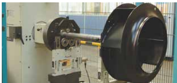
Backward curved centrifugal impellers To prevent accumulation of dirt. Models up to 400 are manufactured from galvanised steel sheet. Models from 450 to 630 are manufactured in sheet steel protected against corrosion by cataforesis primer and black polyester paint finish.
